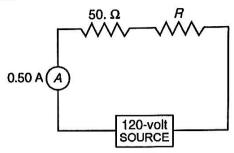
5) Calculate the total resistance of the circuit shown.
